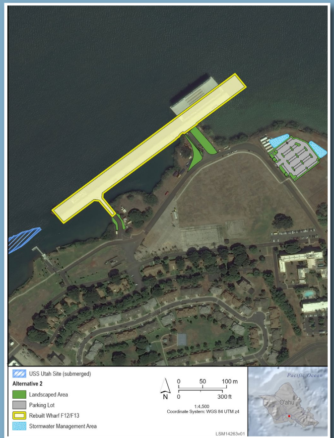
● Figure 2: Comparison of Alternatives 1 and 2. Alternative 1 includes constructing the new LSM home port berth partially within the existing Wharf F12/F13 footprint and shifted northeast along Ford Island, while Alternative 2 includes constructing the new LSM home port berth within the existing Wharf F12/F13 footprint. Alternative 1 provides an additional buffer area between a new LSM home port berth and USS Utah.
