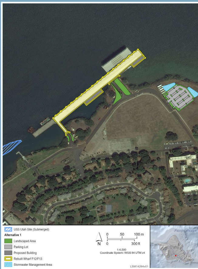
● Figure 2: Comparison of Alternatives 1 and 2. Alternative 1 includes constructing the new LSM home port berth partially within the existing Wharf F12/F13 footprint and shifted northeast along Ford Island, while Alternative 2 includes constructing the new LSM home port berth within the existing Wharf F12/F13 footprint. Alternative 1 provides an additional buffer area between a new LSM home port berth and USS Utah.
